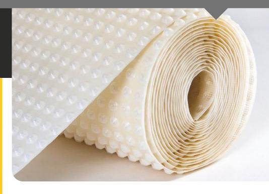
**CM8 Cavity Drain Mesh Membrane** is a 8 mm studded membrane incorporating a tough HDPE mesh lathing welded to the front face, allowing the direct application of various plaster finishes, adhesive 'dabs' and plasterboards and delivering a grade 3 environment to BS8102:2009 and NHBC Chapter 5.4.
