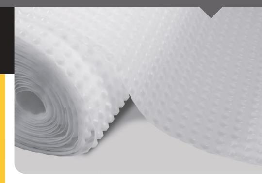
**CM8 Cavity Drain Membrane** is an 8 mm studded membrane, suitable for Type C waterproofing and delivering a grade 3 environment to BS8102:2009 and NHBC Chapter 5.4. CM8 is available in both 500g or 700g densities. We recommend using the CM8 HD700 when a heavier, denser membrane is deemed necessary by the Wykamol Technical Department. Please always take advice from our Technical Experts when making product selections.
